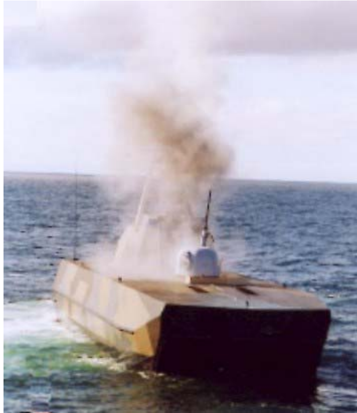
FiReCo has calculated and measured structural responses during gun firing
