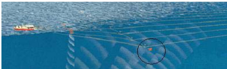
The Barovanes are to be towed from vessels with seismic equipment (Illustration from Baro Mek Verksted brochures)
