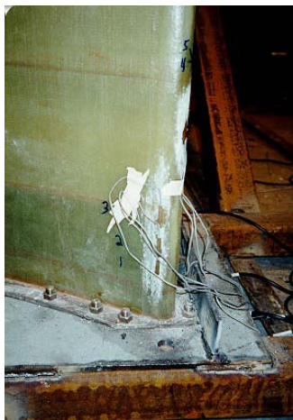
Strain gauges measurement from bending test – early prototype of bonded joint composite foil / steel flange
