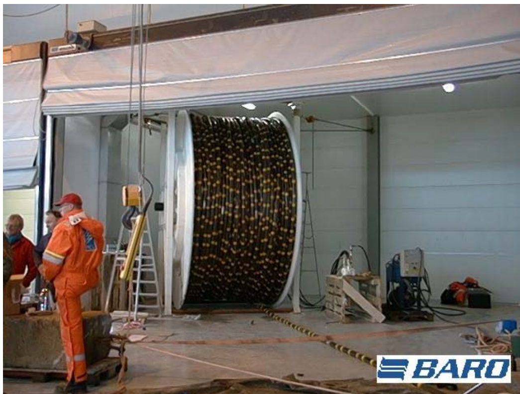
GRP Streamer winch under testing, placed in heat chamber at Baro Mek Verksted
