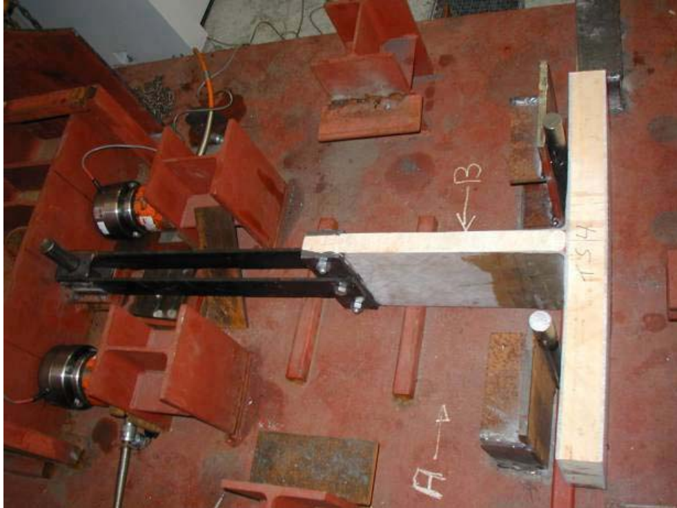
Tensile testing of composite structure internal T-joint
